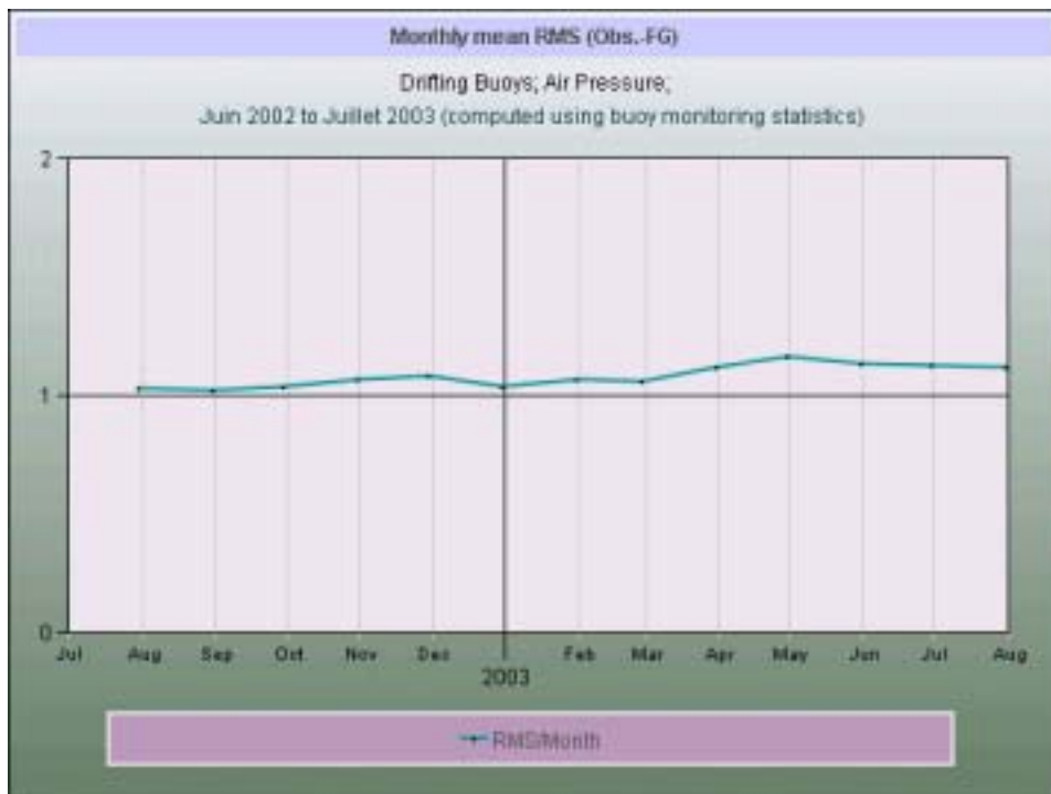
Graph 2: Evolution of mean RMS (Obs.-First guess) per month for the period June 2002 to July 2003 for global GTS air pressure data (from ECMWF monitoring statistics)
