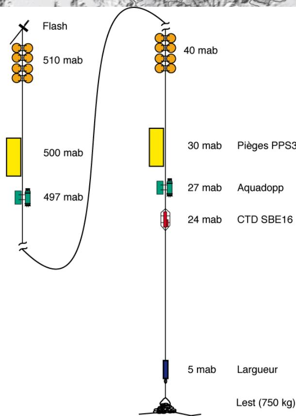
Sediment traps deployed in canyons areas
